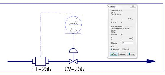
Plus uses its internal PID controller, and in the bottom figure, an external DCS system is used to do the control. Two different layers are used for this on the same drawing.
